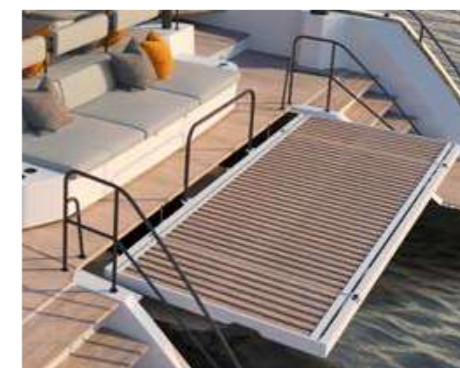
A newly engineered aft platform is capable of lifting a tender of up to 600kg
