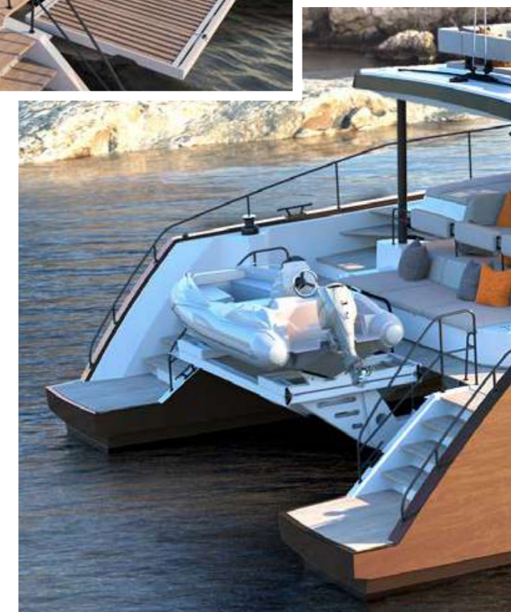
A newly engineered aft platform is capable of lifting a tender of up to 600kg
